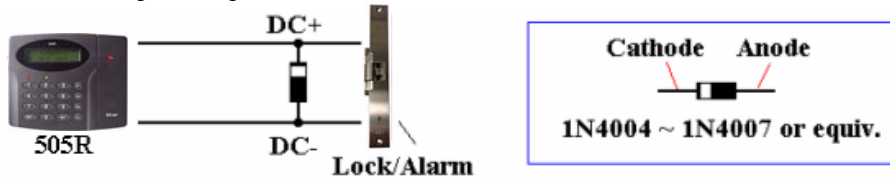
Figure: Reverse Diode connection
